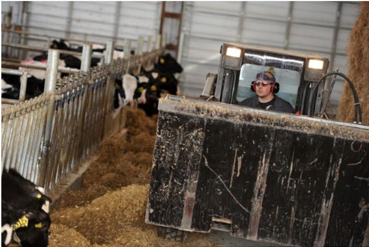
Skid steers are one of a farmer's most useful machines, but they are inherently dangerous to operate. Their power, quick-touch maneuverability and instability when loaded can lead to injury. In addition, the operator's field of vision is extremely limited, which is one of many good reasons to keep young children out of the agricultural worksite.
